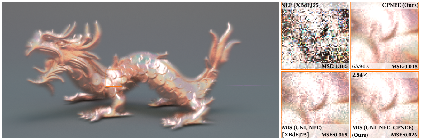
Figure 1: Equal-sample comparison of the dragon scene with a heightfield-like GPIS. The previous NEE method [XBdEJ25] struggles under high anisotropy (top-left inset) since the set of admissible paths approaches a lower-dimensional manifold. Our CPNEE technique importance samples the 1D arc of valid scattering directions restricted to the light’s spherical cap, recovering a clean result in the same number of samples (top-right). Combining all three strategies (unidirectional, emitter NEE, and CPNEE) via multiple importance sampling (MIS) yields robust performance across arbitrary degrees of anisotropy (bottom-right).
